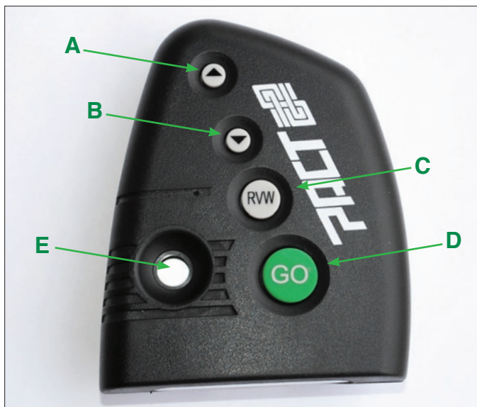
Fig.1 (A) The top of the Club Timer has a "down" button, (B) an "up" button, (C) a "RVW" review button, and (D) a "GO" button. The speaker/microphone is located in the opening (E).
