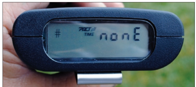
Fig.5 The word none will appear if you press the RVW button and no shots have been recorded (fired).
