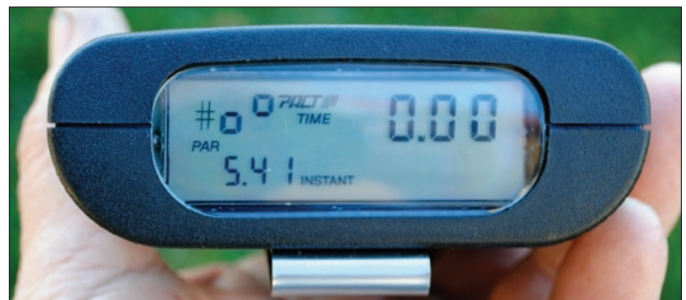
Fig.6 With PAR set, the word PAR will appear on the display along with the PAR time. Here it is set to 5.41 seconds.
