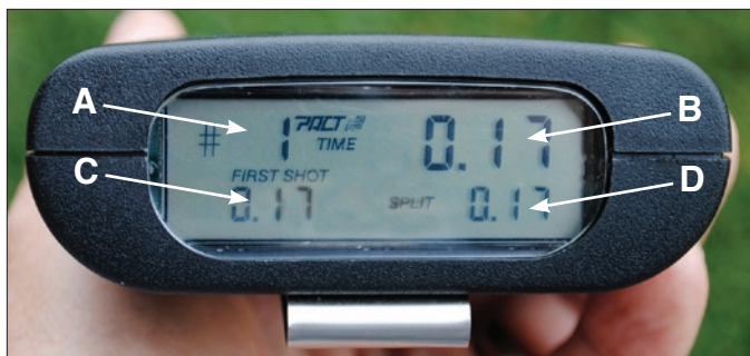
Fig.2 The display shows: (A) sequential number of the last shot, (B) cumulative time since first signal (beep), (C) time from the signal (beep) to the first shot, and (D) the time (SPLIT) between the shot just counted and the previous shot.
