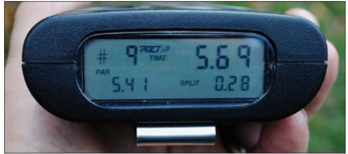
Fig.8 Here the PAR time is still set to 5.41 seconds, 9 shots were recorded over a period of 5.69 seconds. The time between the last shot and the PAR time was .28 seconds (.28 seconds after the 5.41 PAR time setting.)
