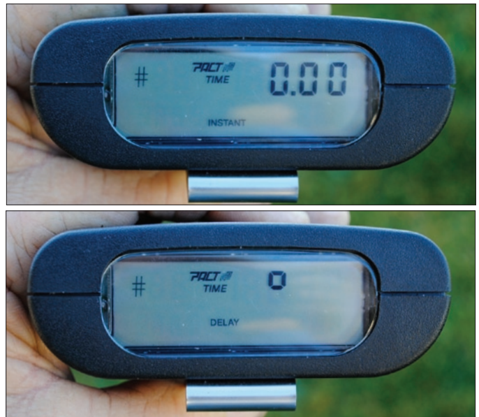
Fig.4 When the unit is set to delay mode, the word DELAY appears on the screen (top photo). When set to the instant mode, the word INSTANT appears. However, either of these words only appears after the button is pressed and before the first shot is counted.
