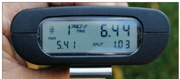
Fig.7 Here the PAR time was run, with only one shot fired. It occurred at 6.44 seconds, 1.03 seconds after the PAR time.
