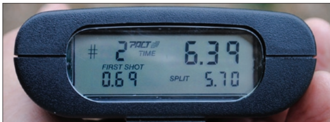
Fig.2 The display shows: (A) sequential number of the last shot, (B) cumulative time since first signal (beep), (C) time from the signal (beep) to the first shot, and (D) the time (SPLIT) between the shot just counted and the previous shot.
