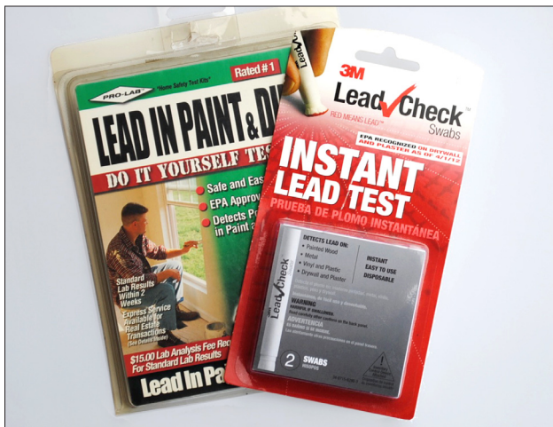
Fig 4. Lead test kits are available at your local hardware store for about $12.00. Depending on the kit, the swabs will allow about four to six tests.
