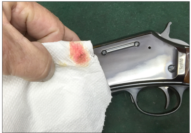
Fig 6. Testing the side frame of this Lightning proved positive for the presence of lead after 60 rounds were fired. The area swabbed was 28” from the muzzle.
