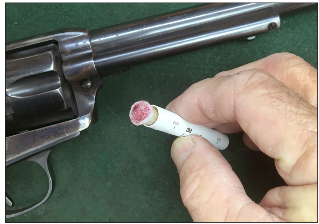
Fig 5. The side of the barrel above the ejector on this SAA proved positive for the presence of lead after only 30 rounds were fired.
