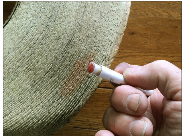
Fig. 1. A lead-test kit was used to determine if the darkened area of the brim of my hat contained any lead residue. When the test kit’s swab turned red, it proved positive for the presence of lead particulate.
