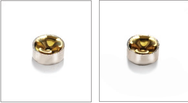
Fig. 6. The anvil in the new CCI primer on the left protrudes from the base of the primer by .010" for an overall height of .119". Once the primer has been installed in a case and compressed (right), the anvil gets squeezed into the cap about .005" but the anvil still protrudes from the base of the primer. (Look carefully at the two primers, the primer on the right has its anvil set slightly lower into the cap.)
