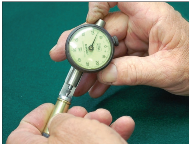
Fig. 2. Primer hits can be measured with a dial micrometer fitted with a special base that measures the depth of the primer's hit below the face of the primer. This primer hit measured .016".
