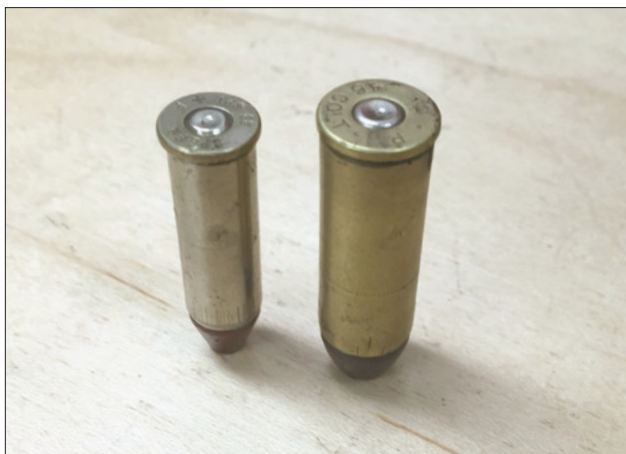
Fig. 1. Both the .38 and .45LC rounds shown here had good primer hits but were ejected from their rifles without detonating. Both had high primers.
