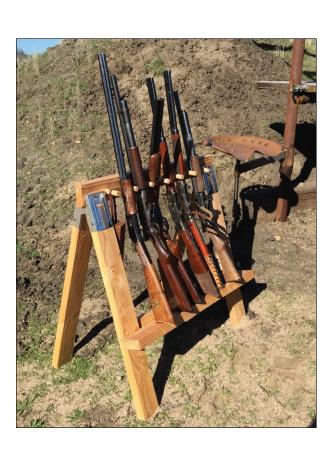
Back stop rail made from 2"x4" cut in half, glued and screwed to 2"x6" bottom support. Stop rail is 26" long.
